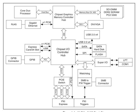
Figure 1-1. NI PXIe-8105 Block Diagram
